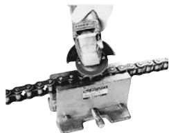
Fig. 2 Grinding the pin ends
