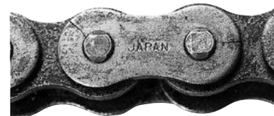
Fig. 32 Hydrogen embrittlement cracking
