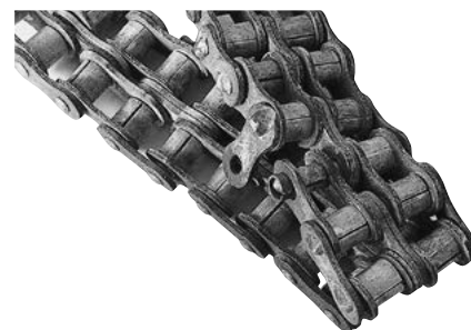
Fig. 31 Corrosion of stainless steel roller chain
